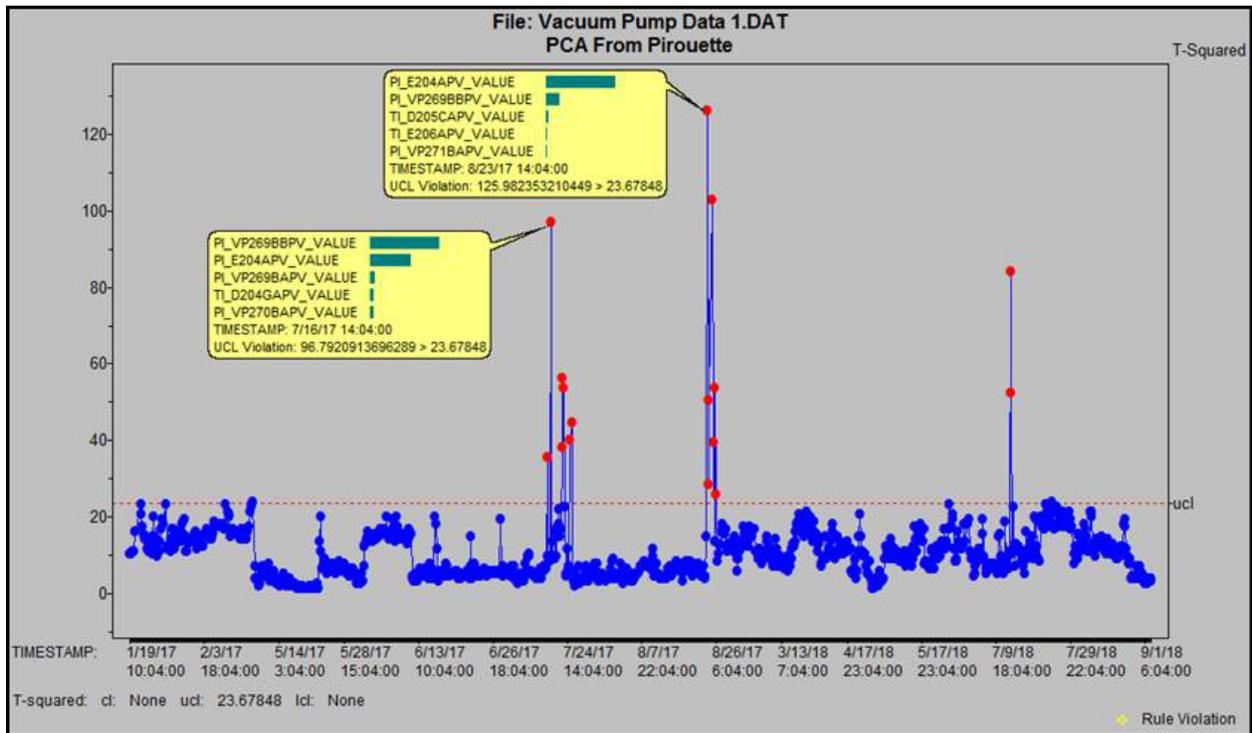
Figure 8. Quality Analyst deployment of multivariate model for vacuum pumps
