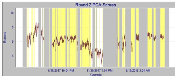
**Figure 2.** Time plot of principal component 1 of all time points when all pumps were on. Gray regions are when pumps were off. Highlighted points (yellow bands) are part of central cluster from Figure 1
