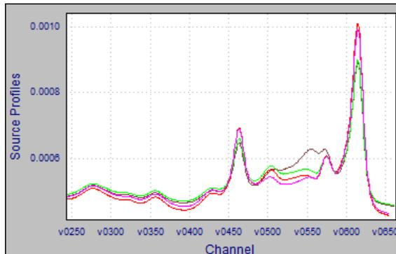
Figure 6. Key Raman shifts during reaction
