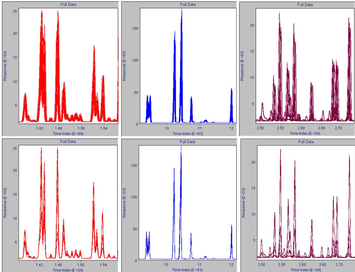
Figure 2. An overlay of 25 consecutive naphtha (red), alkylate (blue) and reformate (brown) runs prior to alignment (top) and after alignment (bottom)
