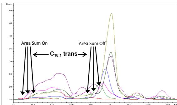
Figure 1: Retention times in several chromatograms have changed such that peak start and end marks cannot be set with confidence
