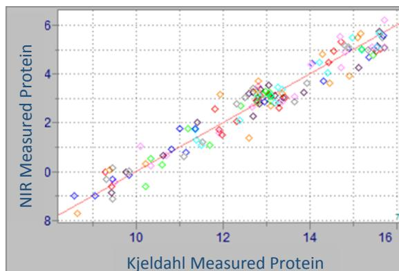
Figure 2. Compositional parameters such as the protein, moisture and fiber content of raw or manufactured food products can be monitored using near infrared spectroscopy and chemometrics
