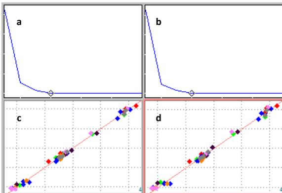
Figure 3. Comparison of PLS and PCR Predictions. (a) and (c) Results from PLS; (b) and (d) Results from PCR; (a) and (b) Variance; (c) and (d) Model predictions vs. octane engine reference values
