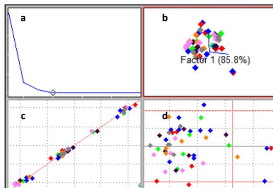
Figure 2. PLS Results for the Octane Data Set. (a) Variance; (b) 3D plot of first three scores; (c) PLS model predictions vs. octane engine reference values; and (d) studentized residuals vs. leverage values
