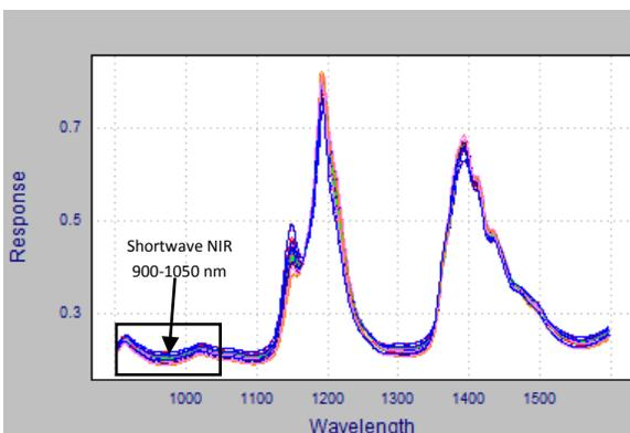
Figure 4. Shortwave region of the near infrared spectra
